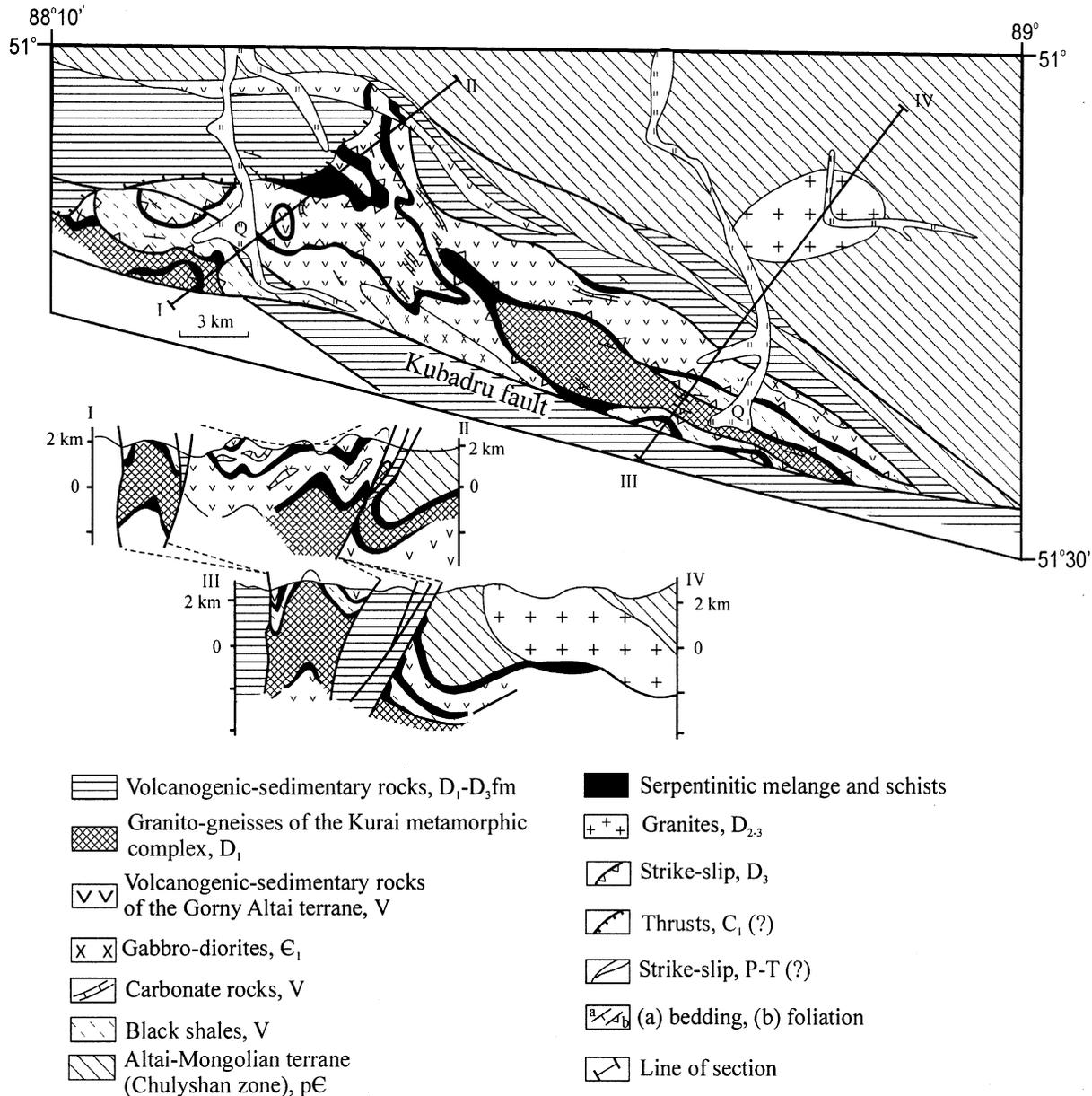
Fig. 8. Geological sketch of the Kurai strike-slip fault which destroyed the  $D_3$  thrust structure at the base of the Altai-Mongolian terrane.
