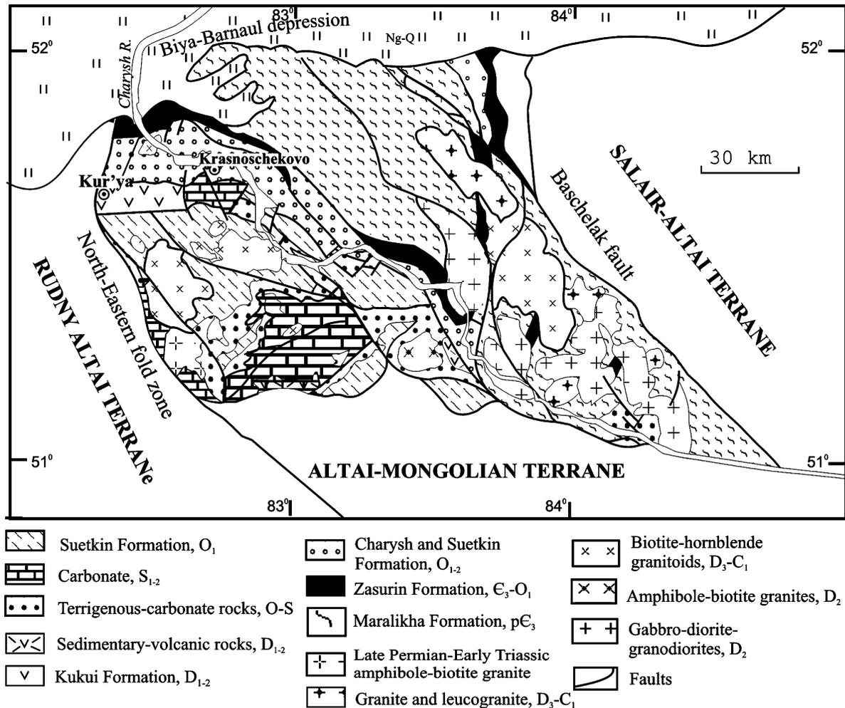
Fig. 5. Geology and structure of the Charysh–Terekta strike-slip zone—Charysh-Inya section in the north-western Gorny Altai terrane (modified from Iwata et al. (1994) and Vladimirov et al. (1997)).
