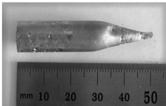
Fig. 2. A \text{Bi}_2\text{Te}_3 crystal grown by the modified vertical Bridgman method with a rotating heat field.
